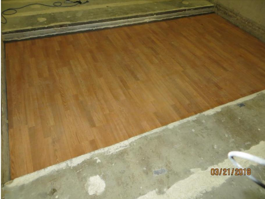
Figure 1 – Specimen mounted in test opening
